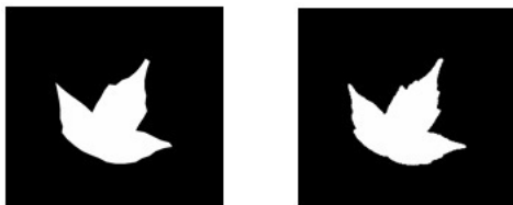
Figure 5. Region boundary points downsampled to 50 points (left) and the original region with 7553 points (right)
